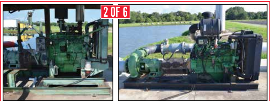
(6) JOHN DEERE Diesel Engines w/CORNELL Centrifugal Pumps
